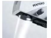
Two-way illumination Shadows in deep channels and cavities are minimized with the two-channel xenon illumination of the surgical microscope.
